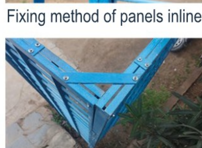
Fixing method of panels in right angle
